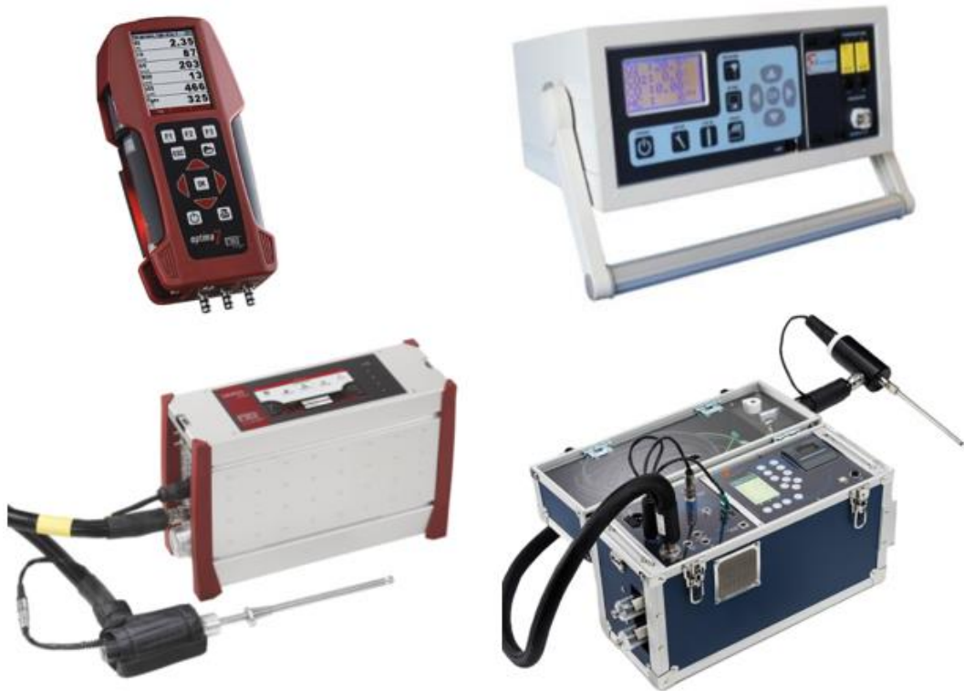
Figure 6 Overview of different type of portable NO x analyzer [10] [11] [12][13]
