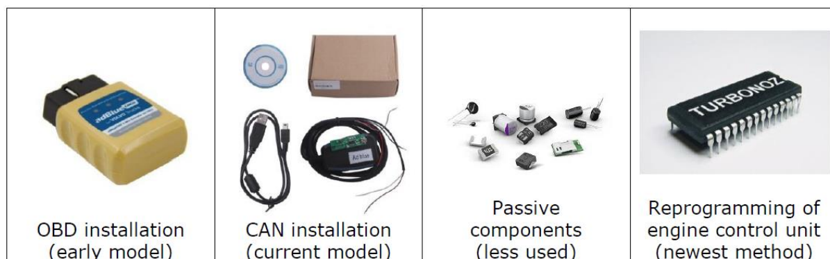
Figure 3 Overview of the four main types of AdBlue Emulators [2]
