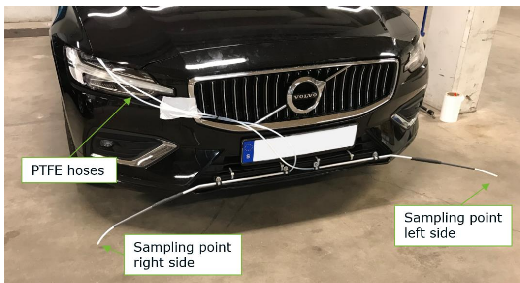
Figure 23 Detailed look of the sampling points/sampling hoses
