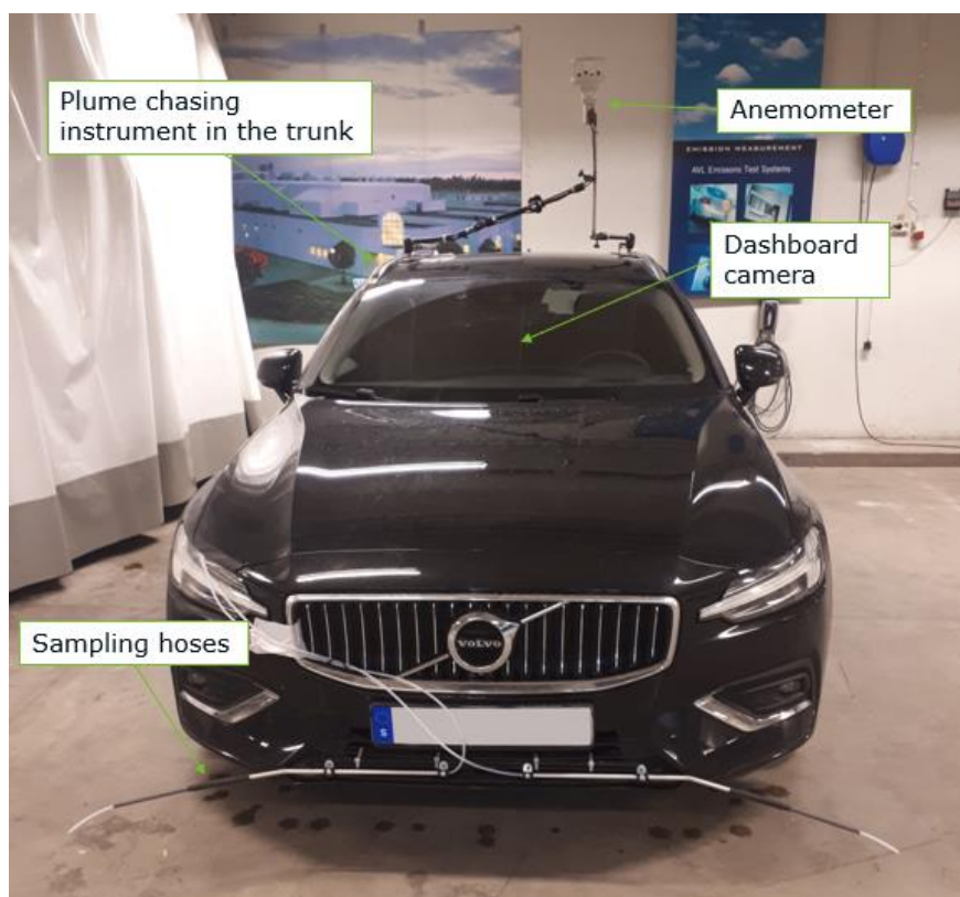
Figure 21 Chasing vehicle equipped with plume chasing equipment
