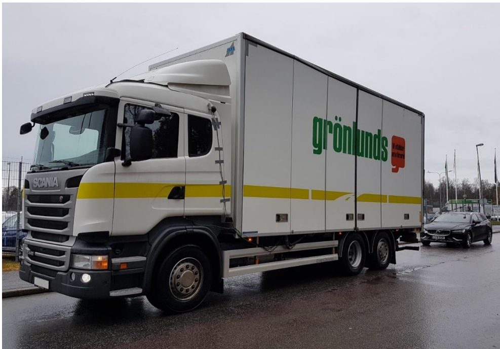
Figure 8 Vehicle 2 - equipped with PEMS equipment and chasing vehicle with plume chasing equipped parked behind. Picture was taking during a short stop along the testing route.
